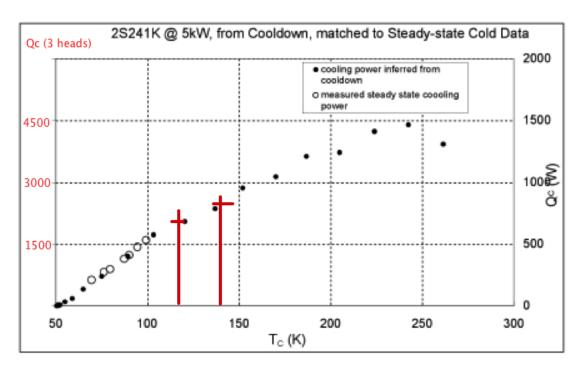
Figure 8: 2s362K Performance Driving (3) 2s241K Coldheads. Left Scale is 3x Single Head
