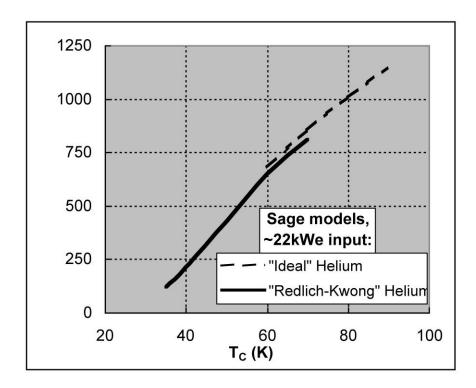
Figure 3: 2s362 Typical Load Curve (single head design available early 2013)
