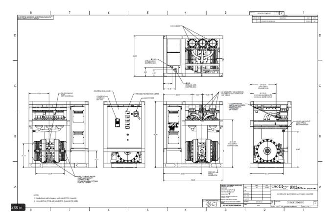
Figure 7: Typical Liquefier Package with Mounting Frame, Drive Electronics and Instrumentation
